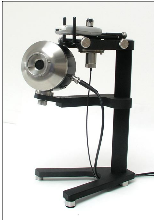
Fig. 1 Telephone Test Head Type 45AA shown here with a Mouth Simulator and Artificial Ear (both available from G.R.A.S.) for testing a mobile telephone
