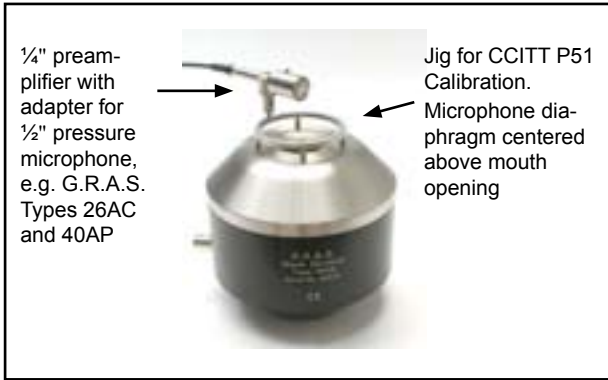
Fig. 2 Setup for calibrating Type 44AB according to CCITT P51
