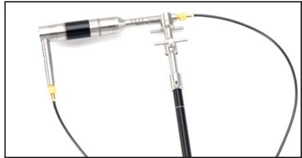
Fig. 2 Sound-intensity Microphone Pair with 25-mm spacer mounted on Intensity Probe Type 50GI
