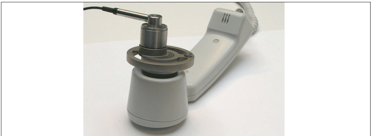
Fig. 4. Place the Ear Simulator centrally over the earpiece of the telephone
