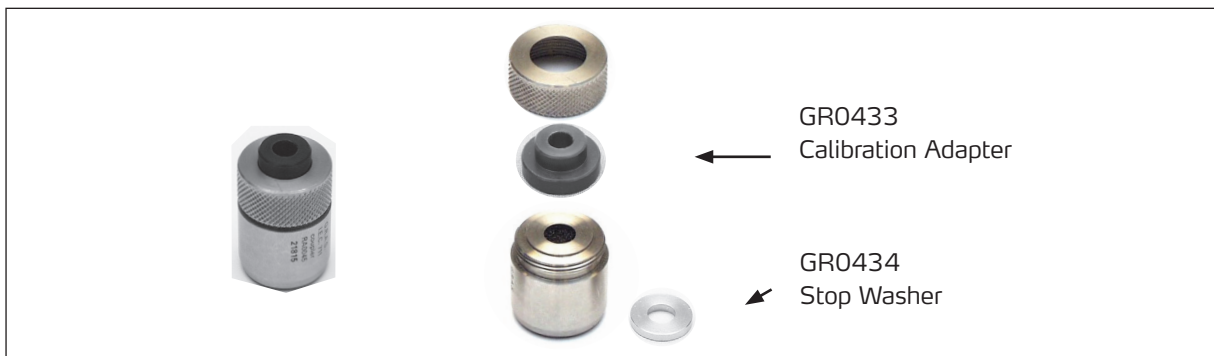
Fig. 12. Assembled and exploded views of the coupler itemising user-serviceable accessories for individual calibration
