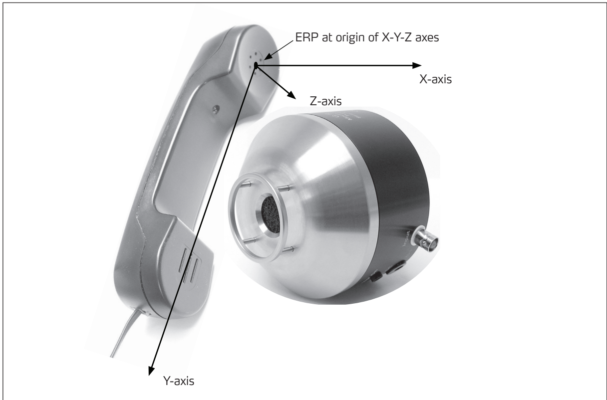
Fig. 7. Showing the basic configuration for testing the microphone of a telephone handset. The ear piece lies in the plane of the Y-Z axes. See Fig. 8 for geometrical details
