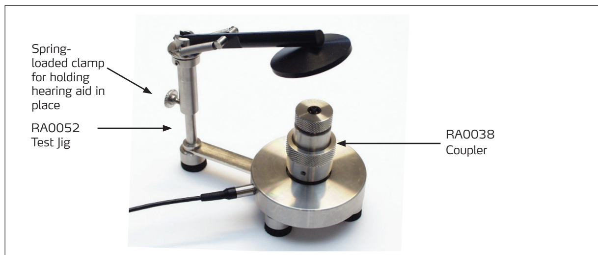
Fig. 1. Assembled 43AB 1/2" 2cc Coupler Kit According to IEC 60318-5
