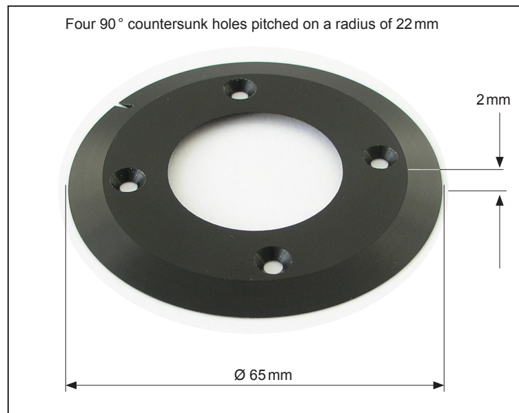
Fig. 7. RA0147 mounting plate for screwing the Surface Microphone firmly in place. It has four 90° countersunk holes, Ø3.2 mm, equally pitched on a radius of 22 mm.
