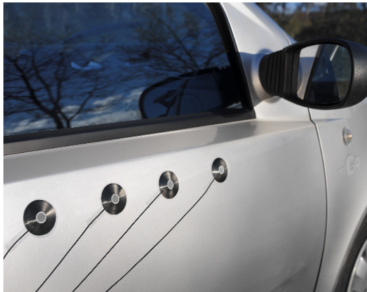
Fig. 5. An array of four Surface Microphones with Fairings (GR0815) mounted on the external surface of a car
