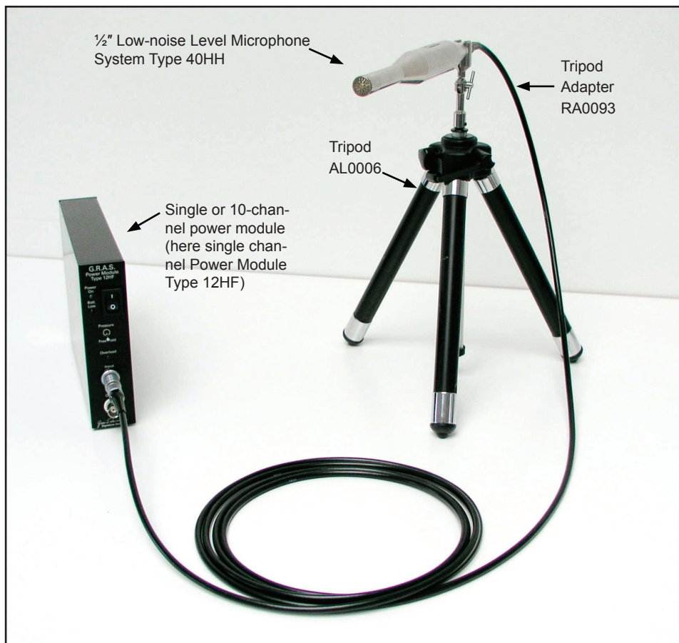
Fig. 1.3 A Single-channel Low-noise Measuring System as described in this document; shown here with Tripod and Tripod Adapter (both available from G.R.A.S.)
