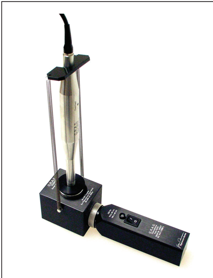
Fig. 3.2 Pistonphone fitted with Coupler RA0090 and the microphone inserted into the Coupler
