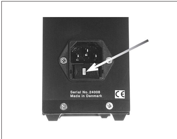
Fig. 3. The voltage setting indicator.
