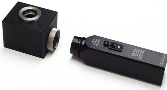
Fig. 3.1 Pistonphone without its normal coupler and ready to accept the Coupler RA0090
