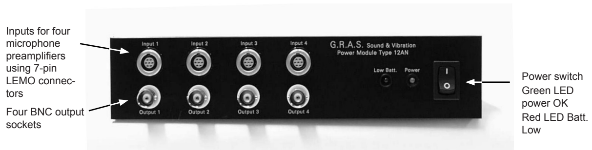
Fig. 2.1 Front panel of the Power Supply Type 12AN
