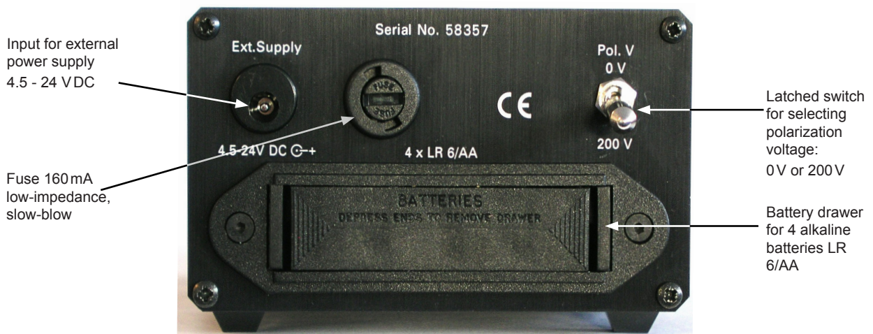
Fig. 2.3 Rear panel of Power Supply Type 12AD
