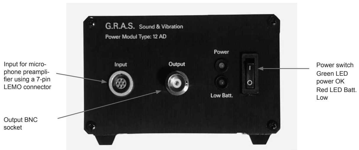
Fig. 2.1 Front panel of the Power Supply Type 12AD
