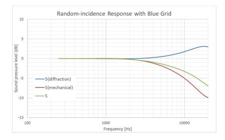
Figure 2 shows the resulting response when the microphone is used in a random incidence field with the blue grid. It is clear from the graph that the resulting response, S, is not flat and the microphone will underestimate the true sound pressure at frequencies above 2-3 kHz.
