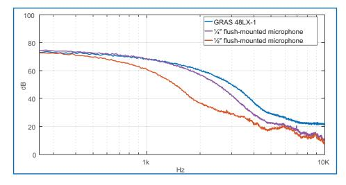
In the case of in-flow measurement where the characterization of the boundary layer is important, measuring with a sensor having a large sensing size will result in a large under-representation of the turbulent high-frequency content. This under-representation is due to the turbulence traveling at the same speed as the flow and having much higher wave numbers that will be averaged sooner.
