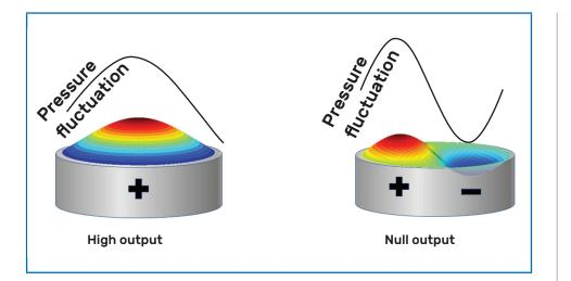
In other words, a sensor with a large sensing element will have a tendency to under-represent the high-frequency content sooner than a sensor with a smaller sensing element (Figure 6).
