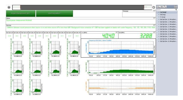
On the left side there are the 10 octave plots of all microphones, on the right you see the three graphs of the result: on top, most important: Sound Power, followed by Sound Level and the correction data.
