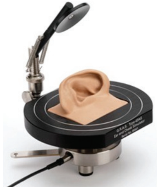
Fig. 3. 43AG Ear and cheek simulator
