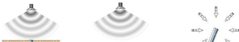
Figure 1. Left: Pressure microphone mounted in an enclosure with an angle of zero degree relative to source. Middle: Free-field microphone in an angle of zero deg relative to source. Right: Random incidence microphone with illustration of sound coming from all directions
