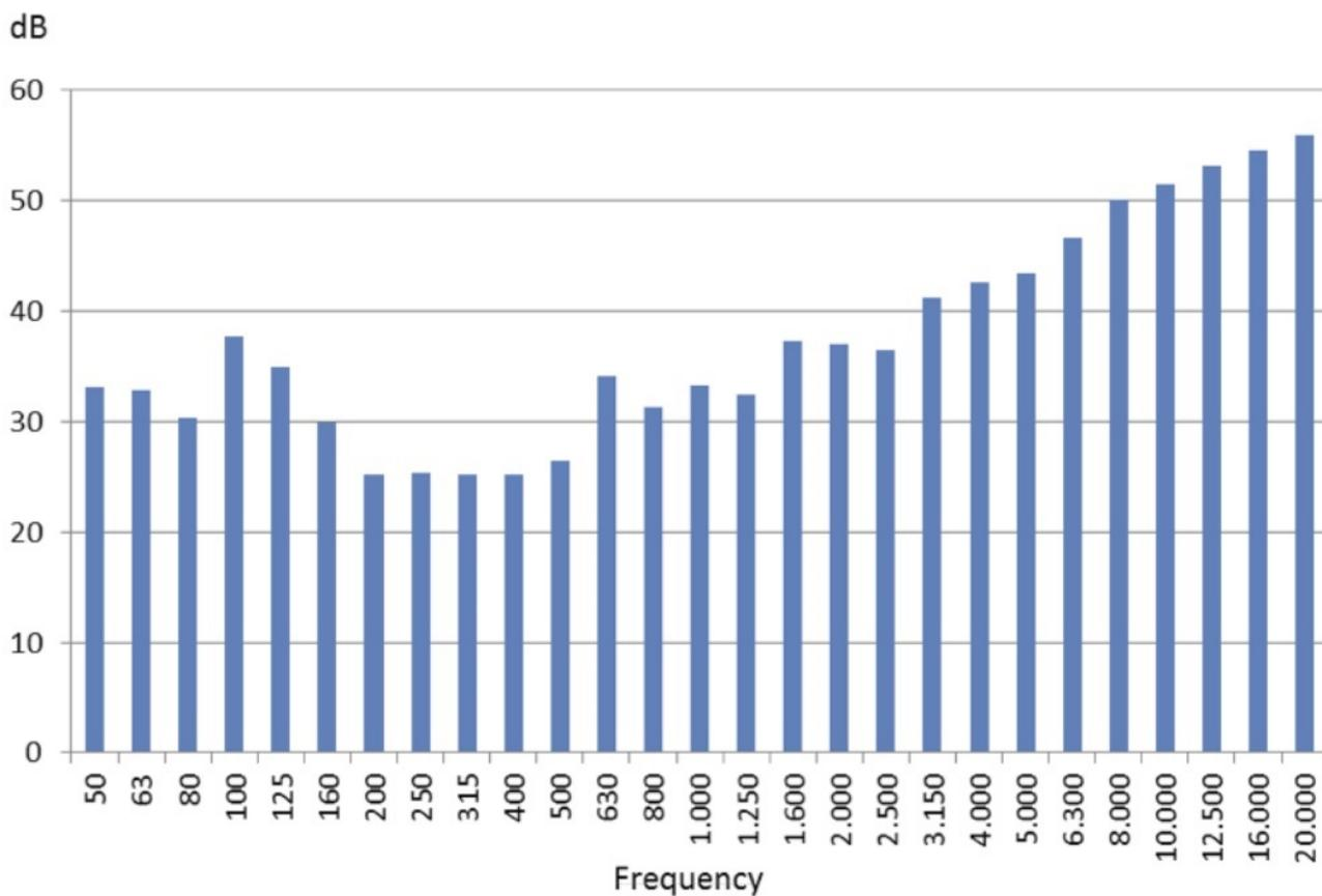
Self Insertion Loss measured in reverberant conditions
