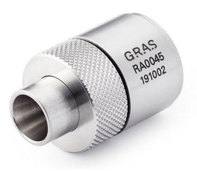
Standards: IEC 60318-4 (based on), ITU-T P.57 Eff vol: 1260 mm<sup>3</sup> @ 500 Hz Res freq: 13.5 kHz ±1 kHz The GRAS RA0045-S5 Ear Simulator is an ear simulator with an acoustic input impedance closely resembling that of an average human ear. The RA0045 includes a 40BP pressure microphone and each RA0045-S5 is individually calibrated with this specific microphone.
